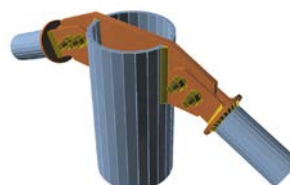
Connecting plates, notches
